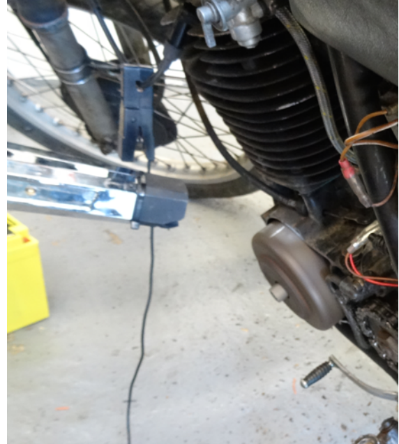
Strobe with inductive clamp attached to HT lead. 'F' mark highlighted in white on flywheel for clarity.
